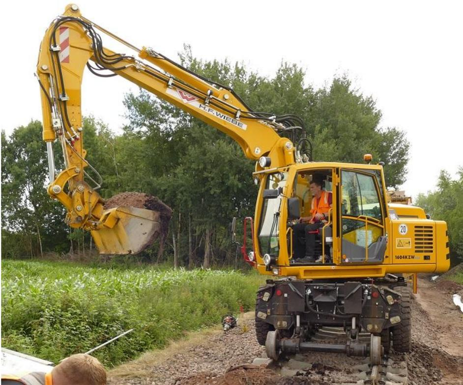
*Image 4: The new double cab – the control center of the 1604 ZW – is perfectly equipped for comfortable and safe operation. This rail-road excavator is a true allrounder and can be operated with 16 different attachment tools, which are adjustable via potentiometer from the cab.*
