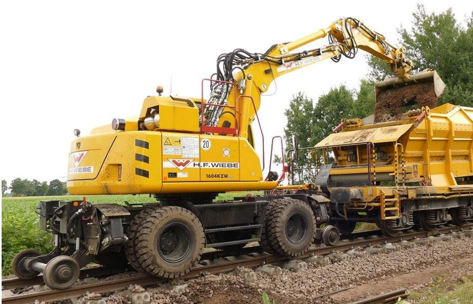
Image 2: In order to extend its reach, this ATLAS rail-road excavator is equipped with a special boom of 3,700mm instead of 3,300mm. Of course, the slewing limitation, operated via an electronic, infinitely adjustable rotation angle sensor, is a standard feature.
