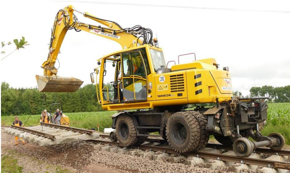
Image 1: Seemingly effortless, the ATLAS 1604 ZW lifts out a track section and places it next to the railroad tracks. The 115 kW/157 hp Tier 4 final engine and AWE4 hydraulic system provide the power and stability for the 22-ton excavator to lift and move weights of up to 15 tons.
