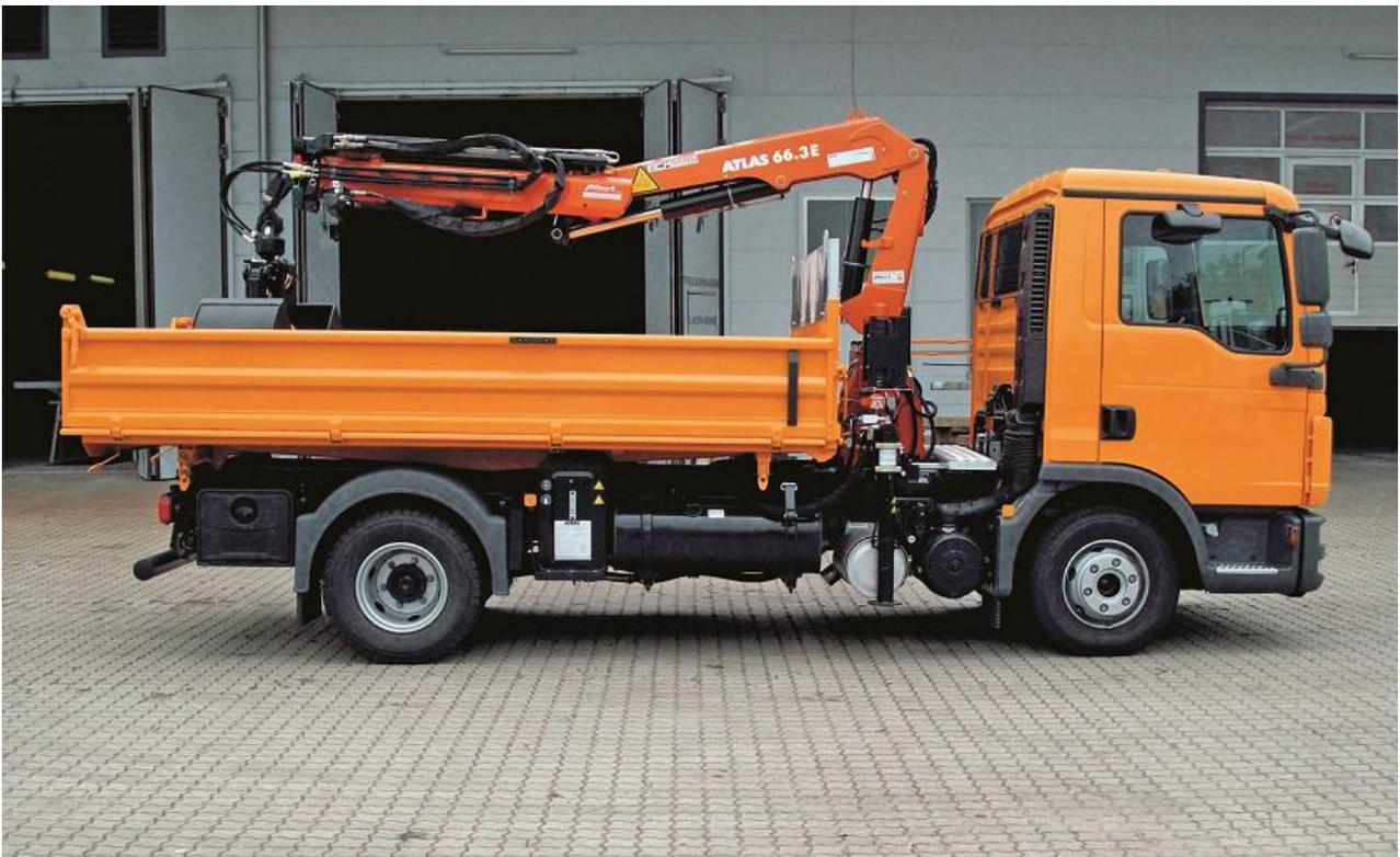
*Image 1: The ATLAS AK 66.3 E – a true all-rounder: a folding crane of the size-class 62 kNm, with up to four extensions, negative boom angle, a maximum reach of 11 m, and a maximum lifting capacity of up to 2.83 tons.*
