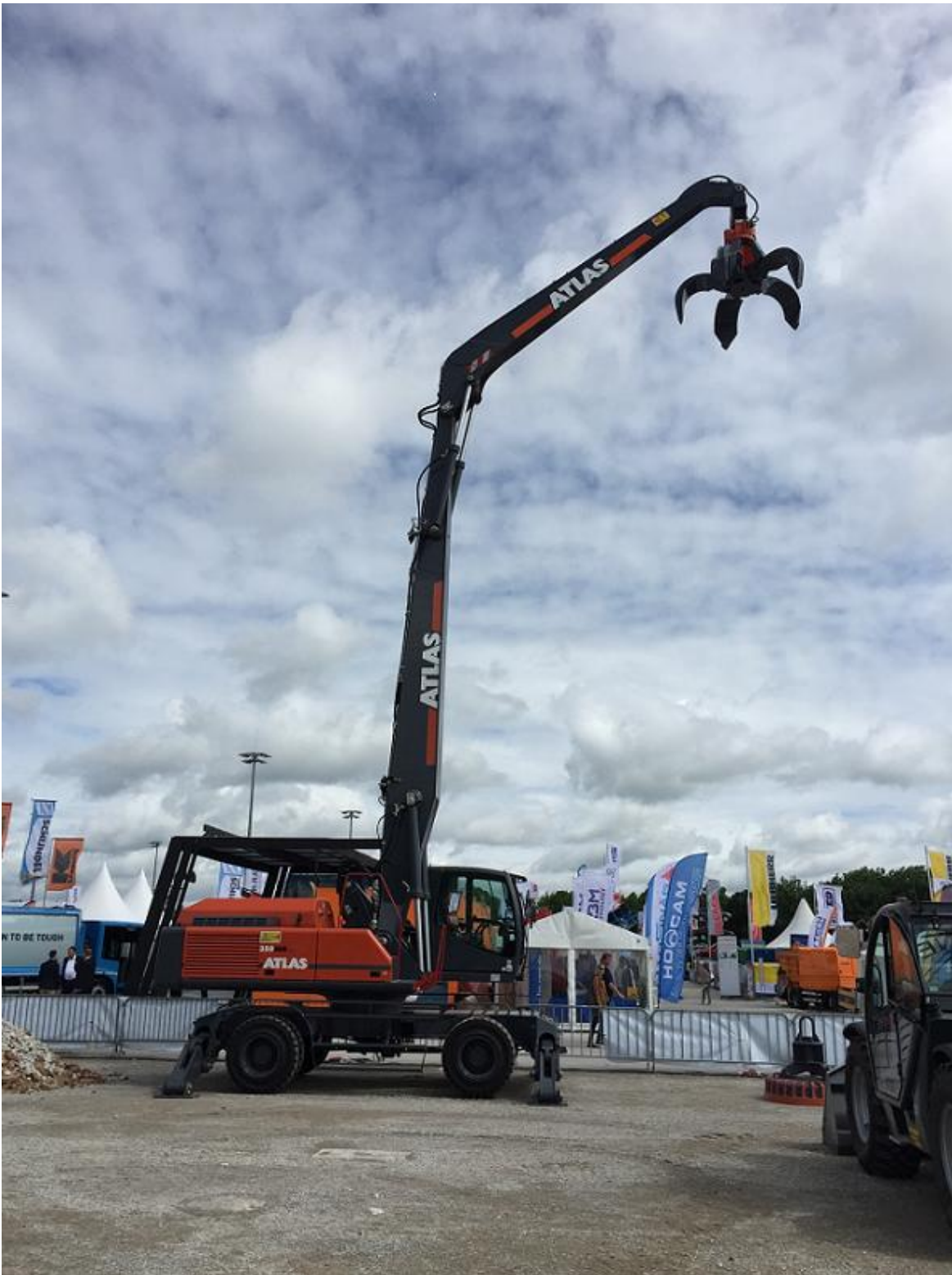
Image 1: The ATLAS 350 MH in the Tier IV final version, equipped with an orange peel grab, at work at IFAT 2016.
