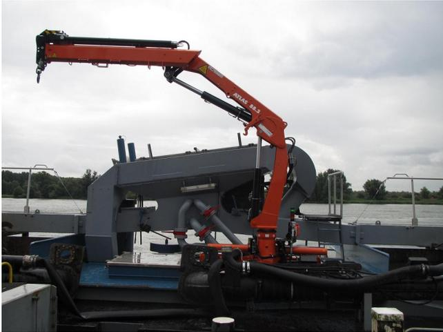
*Image 5: Loader crane as a "stationary installation" working on a boat in the Netherlands*
