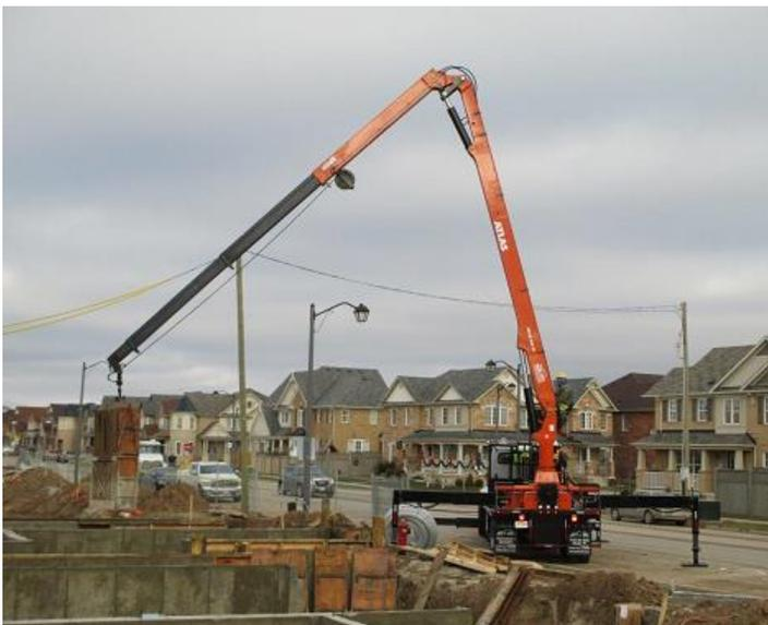
*Image 3: The big solution: ATLAS long reach V-boom crane 440 V with an outreach of 22 meters*
