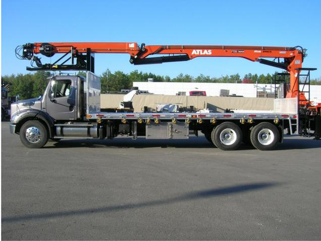
*Image 2: ATLAS V crane, fitted with top seat controls to provide the crane operator with an optimum position.*
